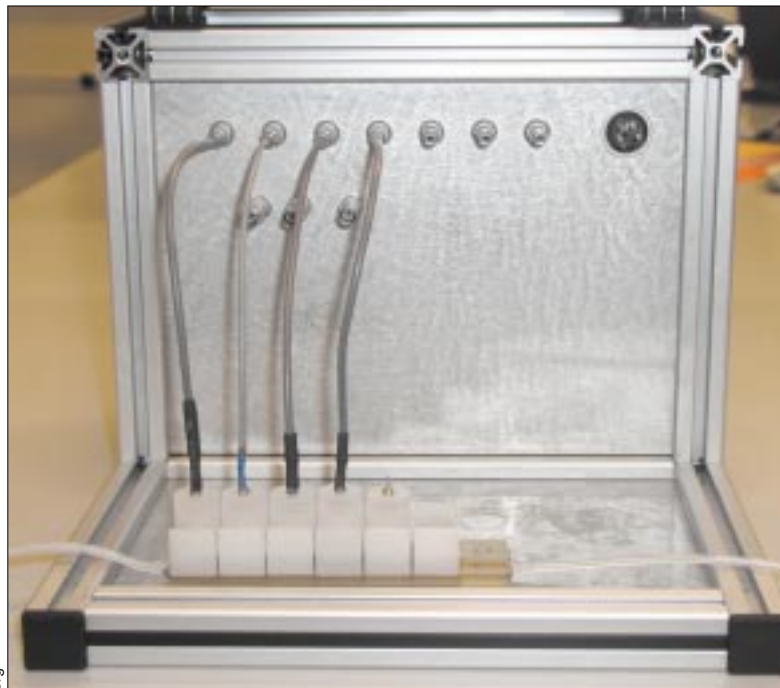
Fig. 3: The present state of the Lab in the Bag®. The picture shows a box with the connectors for six potentiometric, one amperometric channels in the background. A small flow-through system with four potentiometric electrodes is shown in the front. For both measuring techniques a special reference electrode was designed. The box is connected to a lab-top for data processing.
