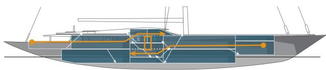
The overlap of the saloon deck (extending from the stern) and the cabin deck (extending from the bow) in the middle of the vessel, in conjunction with the side entrance in this area provide a dynamic structure.
